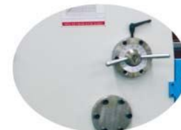
刀片间隙调节手轮 Manual Balde Gap Adjust Wheel
